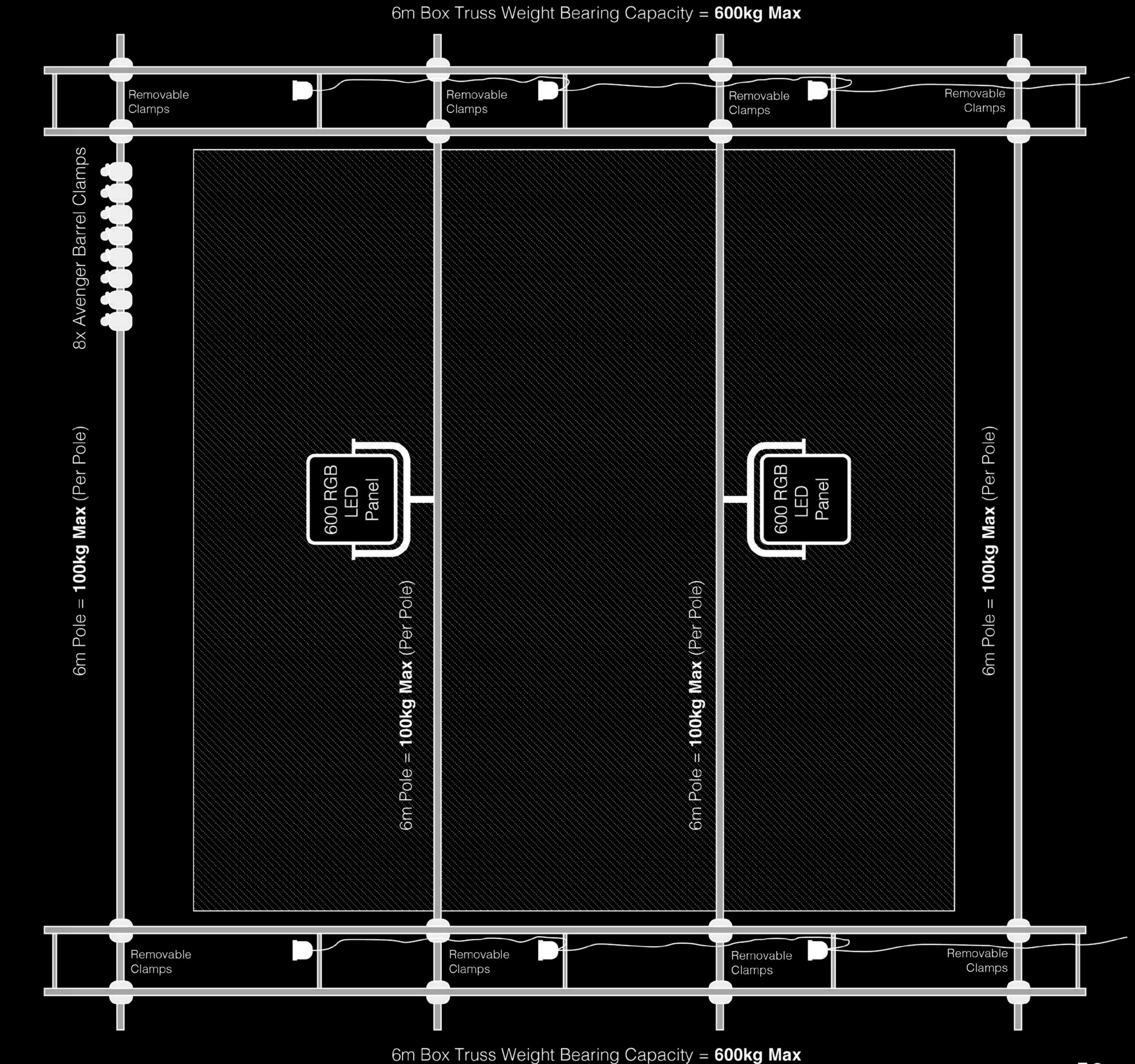
6m Box Truss Weight Bearing Capacity = **600kg Max**
